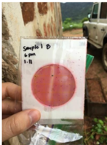
Figure 10: Example of a Petrifilm Test with both E. coli (blue CFU) and Coliform (red CFU) present. This is a test result from Mukaravadanda.
