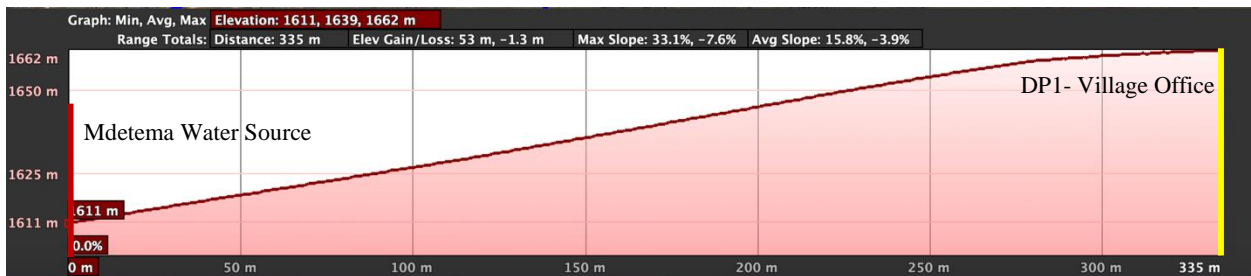
Figure E4: Elevation profile for the pumping pipe from the Water Source to the Village Office.
