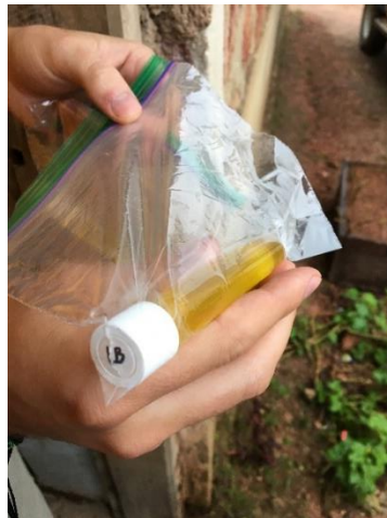
Figure 9: Example of a Colilert Test positive for Coliform bacteria. This is a test result from Mukaravadanda.
