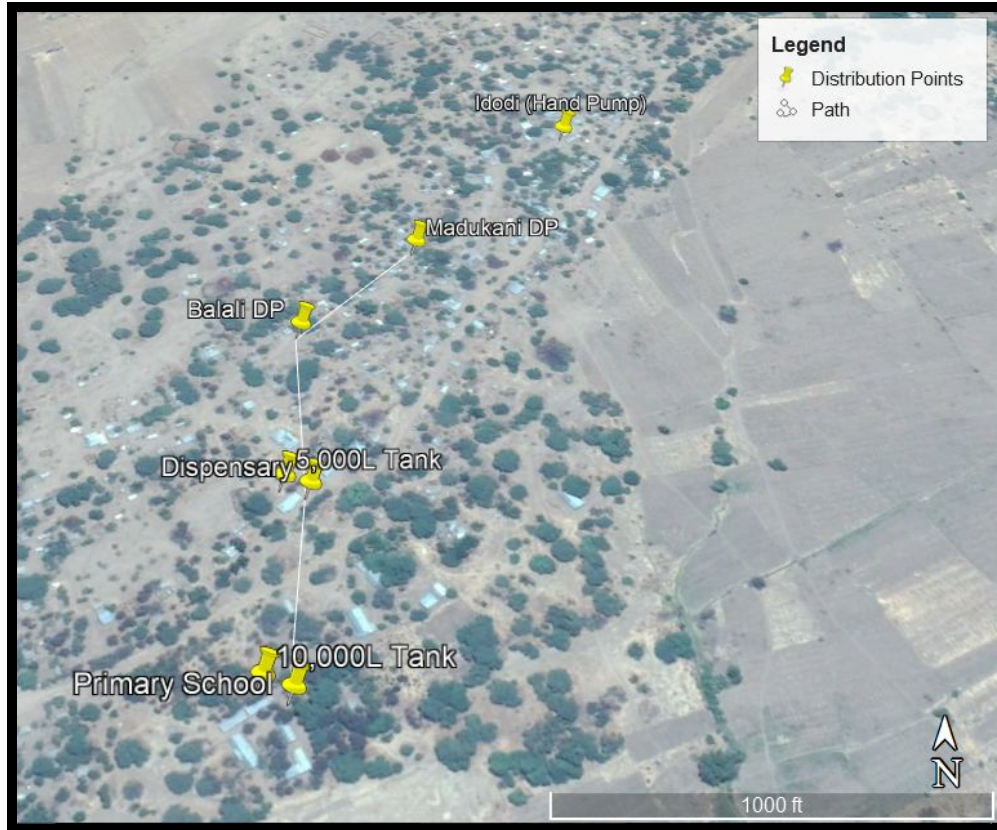
Figure 5.1: Map of drilling locations and distribution points for the first phase of the two-phase system. (Google Earth, Becky Nelson January 2018)
