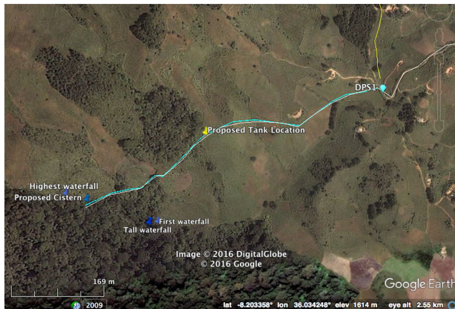
Figure 5.2: A screenshot from Google Earth shows a blown up view of the area in the red box in Figure 5.1, the main gravity line. Multiple points along the mountain stream are labeled, and the cistern could be built at any point where the ground is relatively flat and hard. The pipe line splits into two branches right before DPS1.
