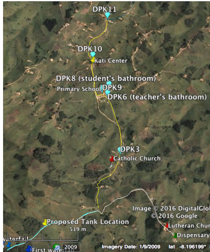
Figure 5.4: The Kati branch of the system, which is the area in the green box in Figure 5.1. The six distribution points and important landmarks are labeled for reference.
