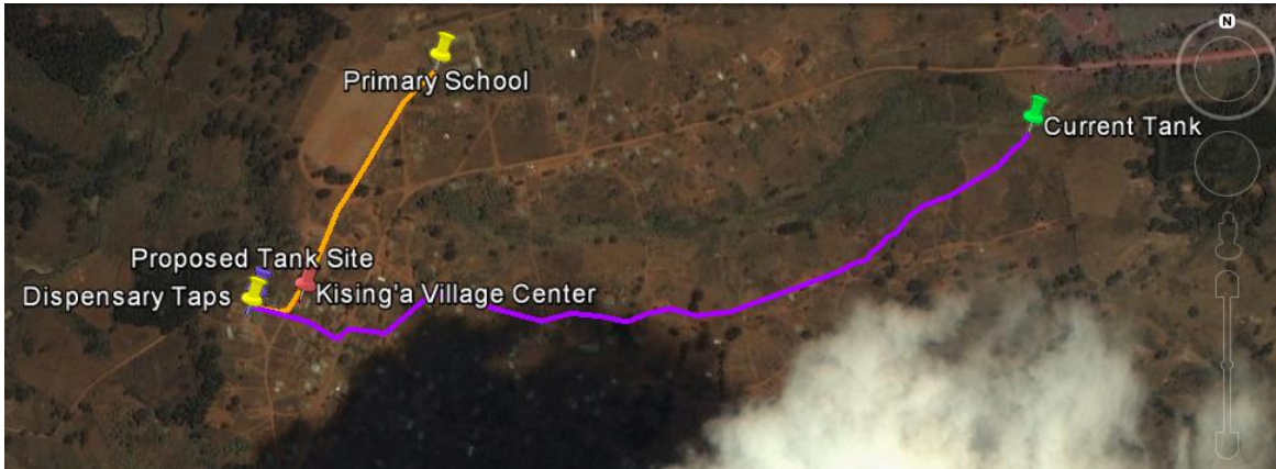
Figure 6 – Overview of the Proposed System. The purple route shows the proposed pipeline from the current tank to the new tank. The orange route shows pipeline from the new tank to the primary school.
