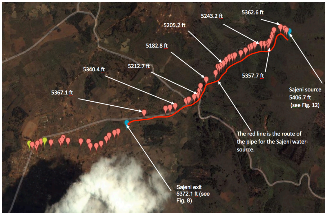
Figure 10: The route of the existing Sajeni line is highlighted in red. From the source of the spring at 5,407ft to the outlet at 5372 feet, there is a 35-ft elevation drop. The outlet would serve the people of Kibaoni.
