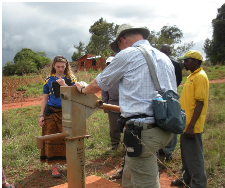
Figure 3: Afridev hand pump near the dispensary that is unusable (GPS Coords: 08° 04' 42.7", 035° 49' 42.9")
