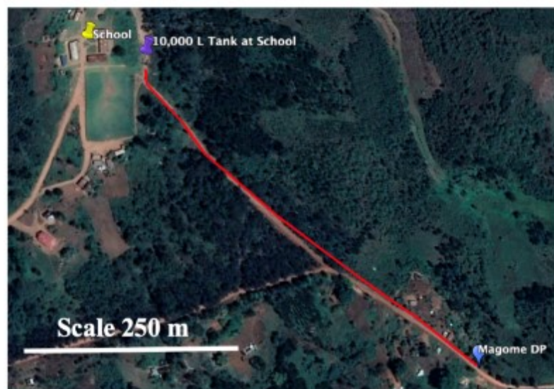
Figure 5.13 | Google Earth View of Magome Line. Location of the primary school (yellow), the location of the 10,000 tank (purple), the line running to the DP (red), and the Magome DP (blue).
