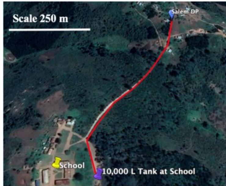
Figure 5.12 | Google Earth View of Salem Line. Location of the primary school (yellow), the location of the 10,000 tank (purple), the line running to the DP (red), and the Salem DP (blue).
