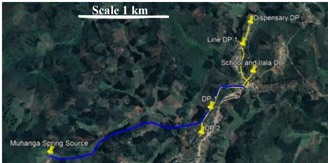
Figure 5.7 | Overhead View of the Proposed Phase I System. Note that the blue line represents the gravity main, whereas the yellow lines are supply lines to DPs.
