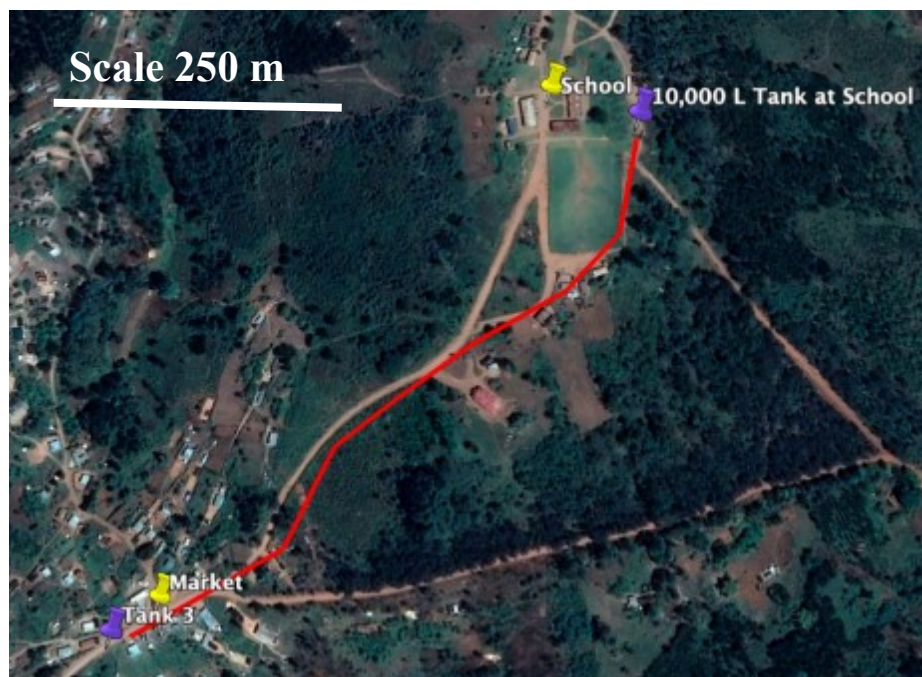
Figure 5.10 | Google Earth View of Pumping Line. Location of the market and primary school (yellow), the tanks located in the market and at the school (purple), as well as the pumping line connecting the two tanks (red).
