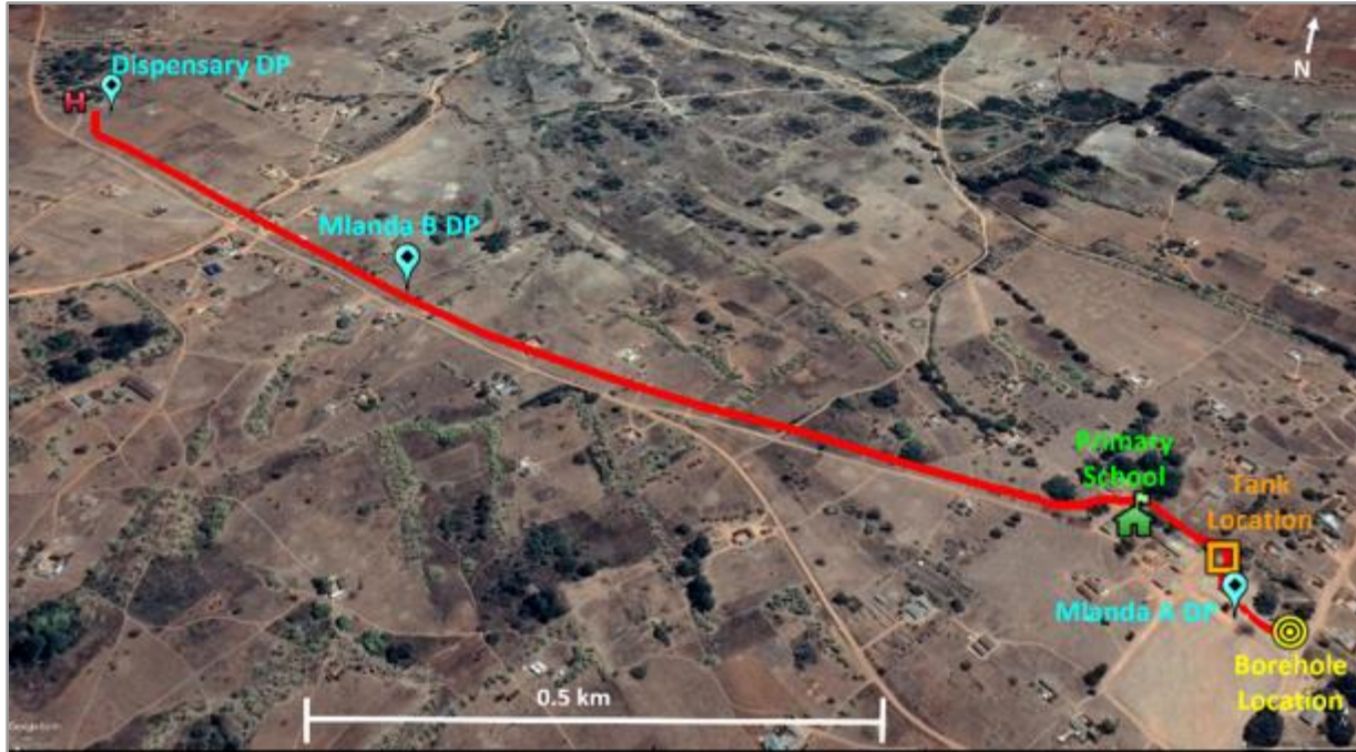
Figure 5.7: This Google Earth screenshot depicts the Phase II water delivery system. The three DPs are marked in light blue. The system starts at the pre-existing borehole marked by the yellow target and fills the nearby tanks adjacent to the primary school. The gravity fed pipes, marked by the red path, flow out of the tanks, around the primary school, and along the road to the other DPs.
