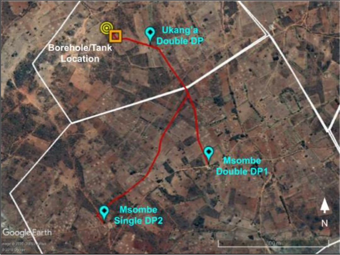
Figure 5.3: This figure displays the paths taken to connect the borehole to the tank to the different distribution points in Ukang'a and Msombe.
