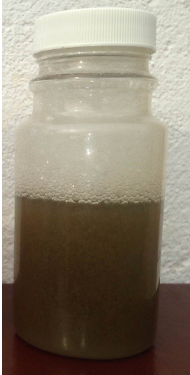
Figure 4: Water Test for a hand dug hole
