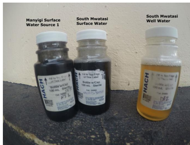
Figure 1.2.3 South Mwatasi Water System. The distribution tap (b) located adjacent to the pump house, supplies water from a 2,000 L storage tank. When the tank is empty, villagers go down to a surface source (a) to obtain water. A water test (c) was performed to determine water quality. Black water indicates bacteria levels higher than what is suitable for potable water while yellow indicates potability.
