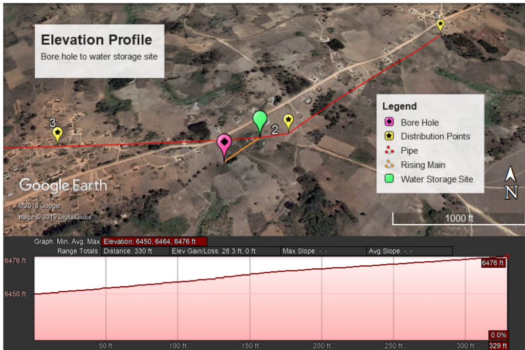
Figure B.1: Elevation profile for proposed borehole location to proposed water storage tank location.
