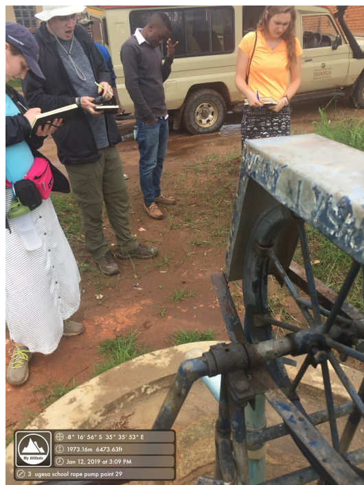
Figure 7: Rope pump dug in 2015 and currently used by students at Mong’a primary school. Well depth is 9.1 m and original water level was 1.5 m. In the wet season this pump fills approximately 15 to 20 buckets at a time and requires 12 hours to refill while in the dry season the pump fills 1 to 2 buckets at a time and requires 24 hours to refill.
