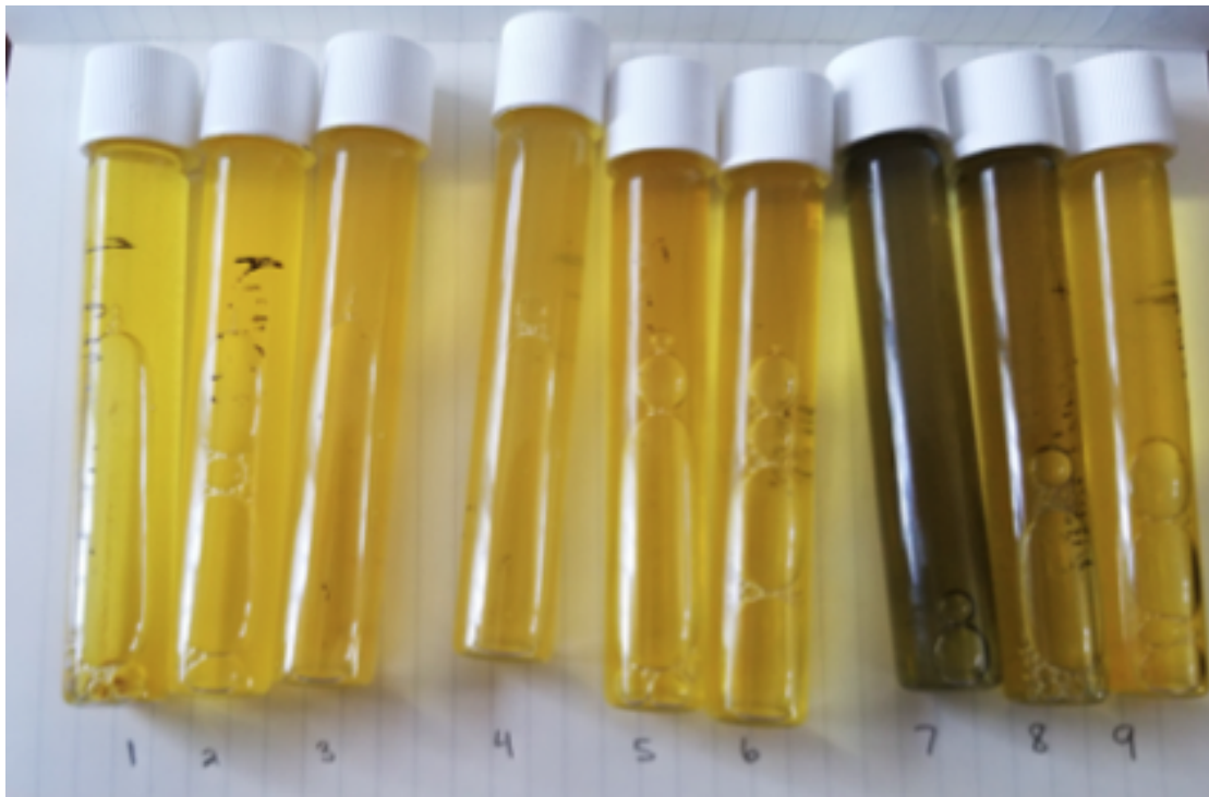
Figure 3.6 Results of Colilert water tests after approximately 24 hours of incubation.
